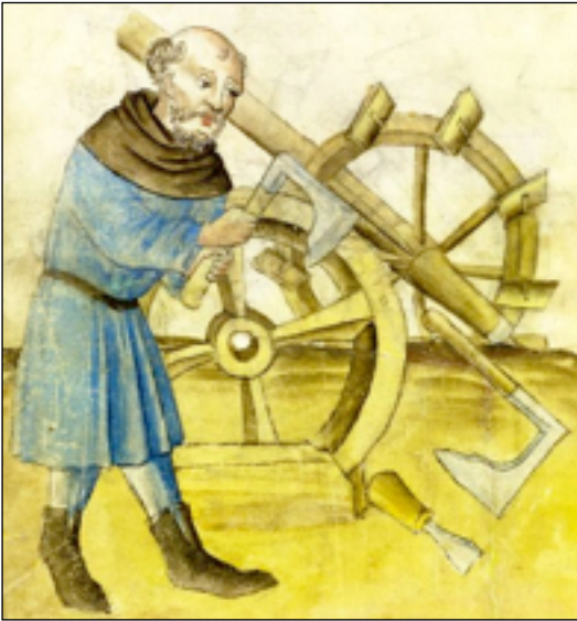
ABBNEY WHEELWRIGHT SHAPING WHEEL RIM WITH AXE. NOTE WATER WHEEL USING SAME BASIC CONSTRUCTION IN BACKGROUND. HAUSBUCH DER MENDELSCHEN ZWÖLFBRÜDERSTIFTUNG, NÜRNBERG, MENDEL I AMB. 317.2° FOL. 87R.
