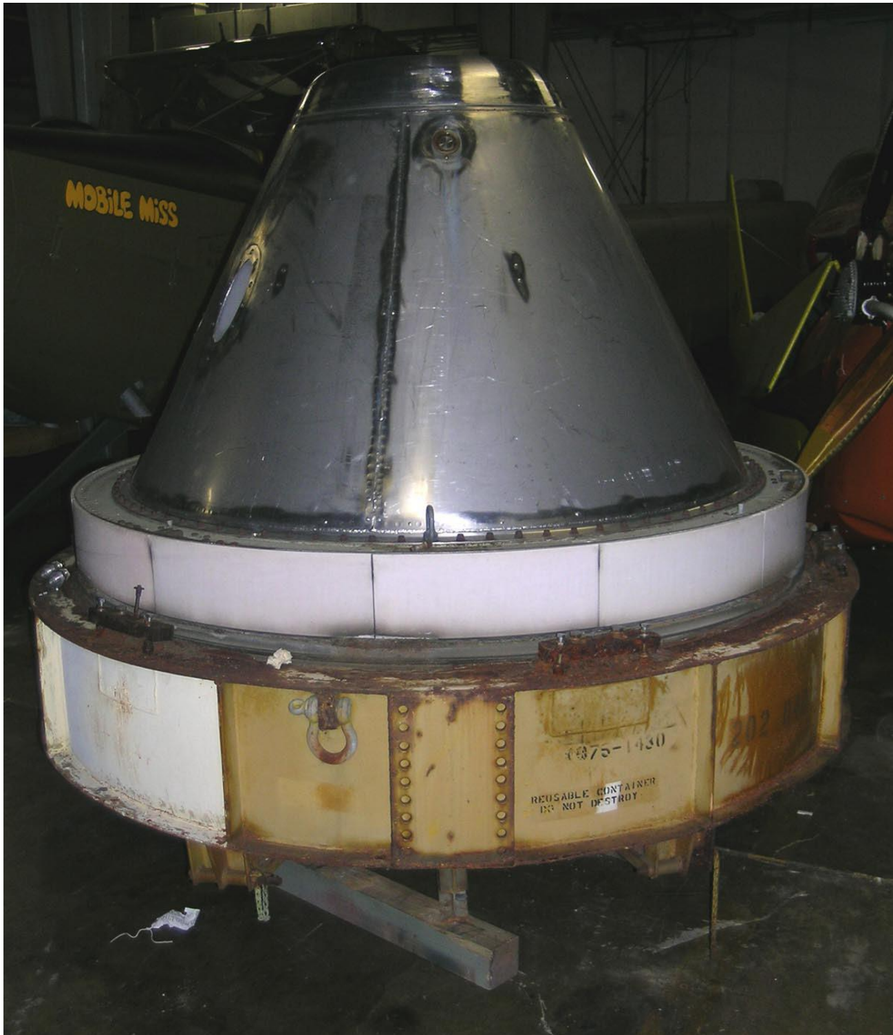
General Electric's Mark II reentry vehicle, which used shockwave formation and a thick copper heat sink to protect the warhead beneath it from the enormous temperatures generated from hitting the atmosphere at speeds of 25,000 miles per hour.
