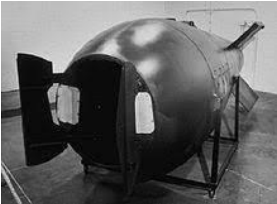
The Mark 5 bomb, designed with clam-shell doors to allow “IFI”—inflight pit insertion. This was SAC’s standard atomic bomb during much of the 1950’s. More than 500 were produced.
